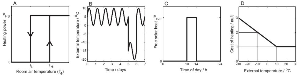
**Fig. 2.** Functions used in the simulations. (A) The heating of the room air was modeled as an on/off-heater with hysteresis. (B) The external temperature was a daily sinusoidal, to which in two cases was added a cold spell every fifth day. (C) Daily free heat was added to the room air at midday in two simulations. (D) In one simulation the cost of heat was modeled as increasing with decreasing external temperature (au/J = arbitrary units per joules of heat).
