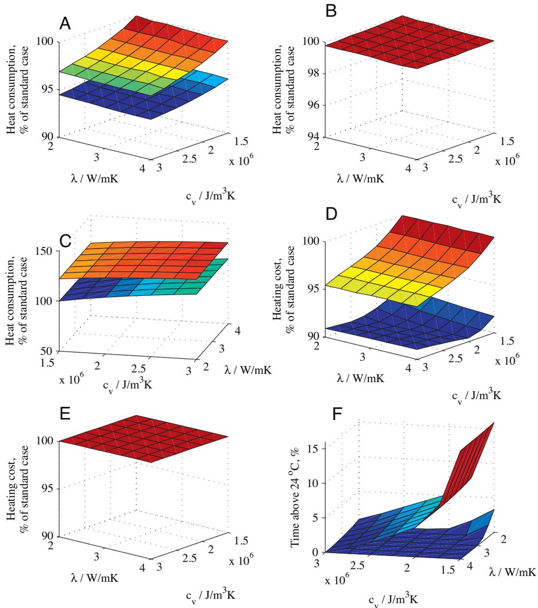
**Fig. 3.** The simulated results in the six cases described in Table 1 and the text. The top surface in each diagram is for a wall thickness of 0.1 m and the lower surface is for a wall thickness of 0.3 m (for (B) and (E) only one surface is shown as the two surfaces are almost identical). Note that the plots have been rotated differently in the heat capacity–thermal conductivity plane to more clearly show each result. The coloring differentiates different levels.
